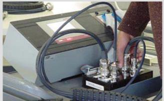
Hipot testing of newly-installed cables is standard on most projects and should be done early on before permanent power is brought into a building. It should only be performed by a qualified professional. Working with high voltage comes with risk of electrical shock, so it is important to use hipot testing equipment that meets current requirements, and to strictly follow all safety regulations and manufacturer precautions.
