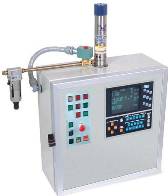
**Many manufacturers have built-in cooling systems** for equipment that generates heat (VFDs, etc.) but custom cabinets may need to have cooling provided, and there are several types available. DX and Venturi systems are sometimes used, but vortex cooling systems are most common. This low-cost method both purges and cools the enclosures using a vortex tube that creates cold air from ordinary compressed air.
